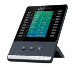
The ZIP 450M's 4.3" 272x480 pixel color screen can add up to 60 additional programmable keys to ZIP 49G phones. Up to 3 expansion modules can be daisy chained per each phone.
